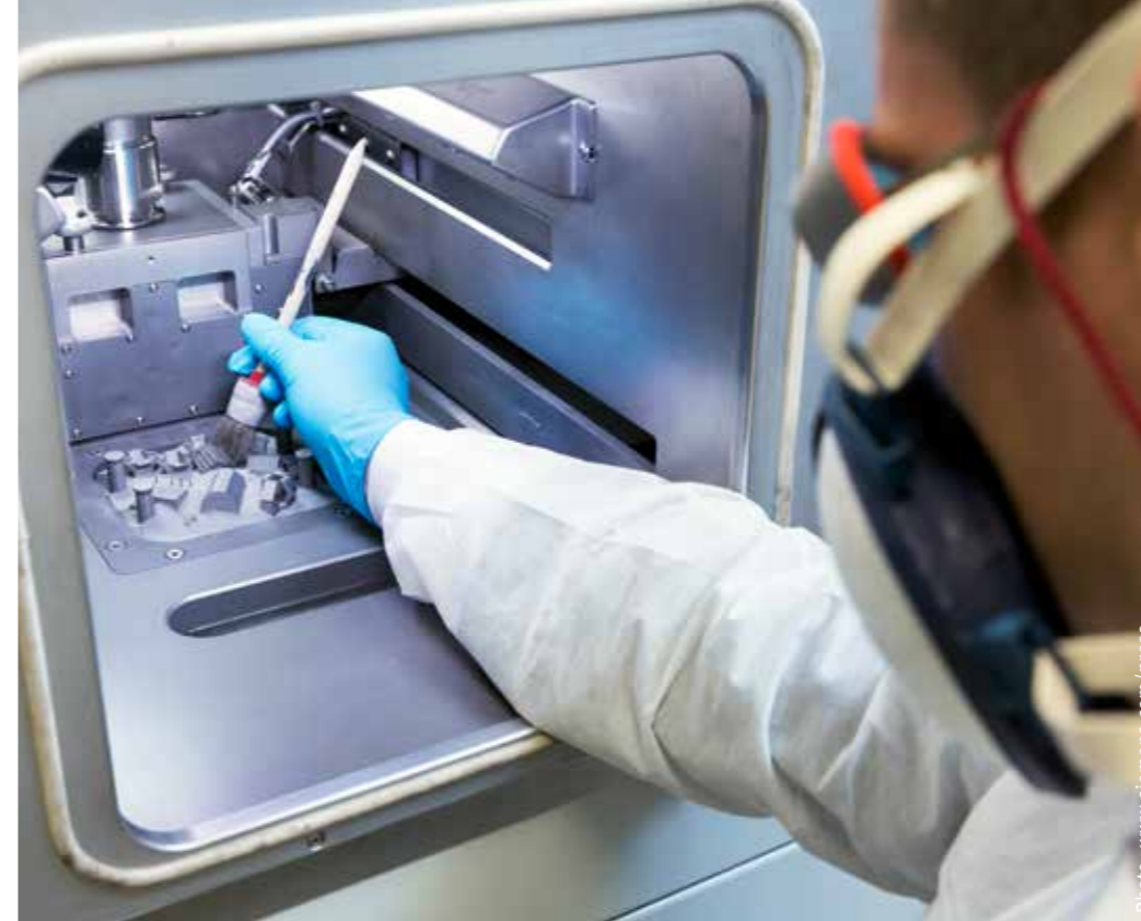
When the printer is finished, large quantities of metal powder are left behind and must be carefully removed.
