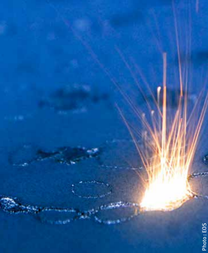
The direct metal laser sintering (DMLS) process used for dental crowns and bridges.
