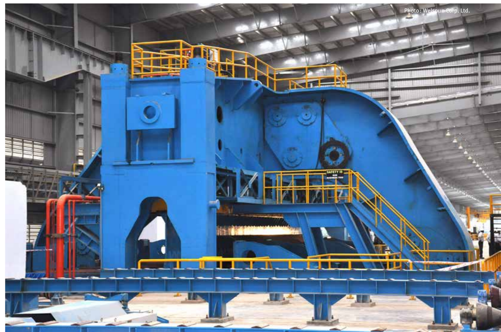
Welspun uses the JCO forming process, which has gained recognition in recent years as one of the most cost-effective and flexible processes for producing high-quality tubes.
