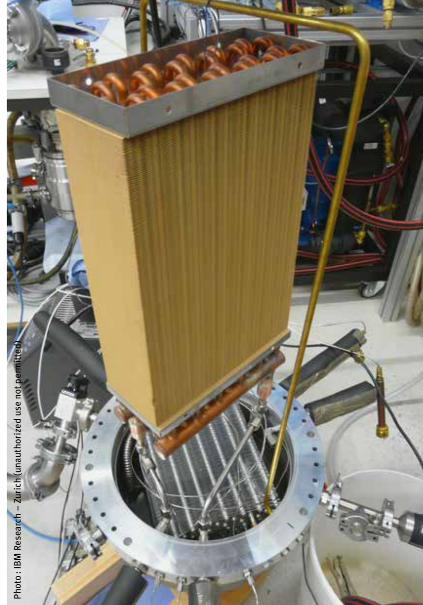
Scientists at IBM Research, Zurich, Switzerland, are collaborating with external partners on a project that might potentially enable cloud data centres of the future to cool themselves using their own waste heat. An adsorption heat exchanger (seen above) will convert heat to cool air using vapour, water and silica gel.
