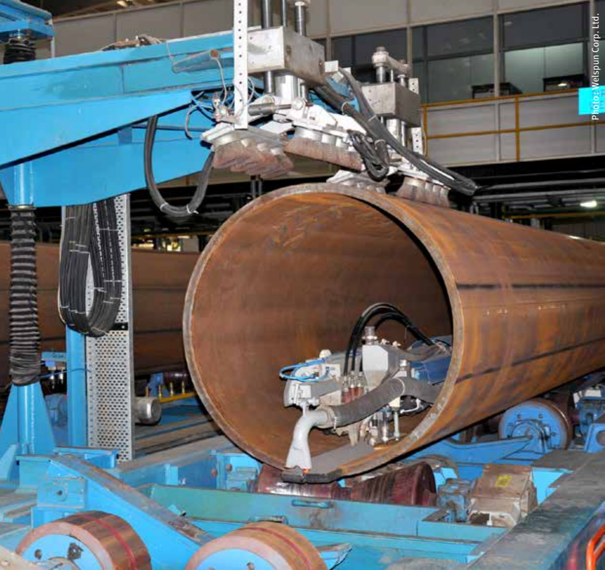
Welspun uses submerged arc welding (SAW) – a welding process that can deliver high deposition rates and deep penetration at a very rapid pace. Here, the interior of Welspun’s SAW.
