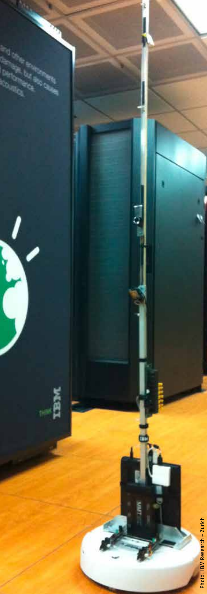
Using IBM's Measurement and Management Technology (MMT), this self-propelled MMT robot generates a heat map that helps pinpoint, diagnose and remedy data centre trouble spots and energy inefficiencies.
