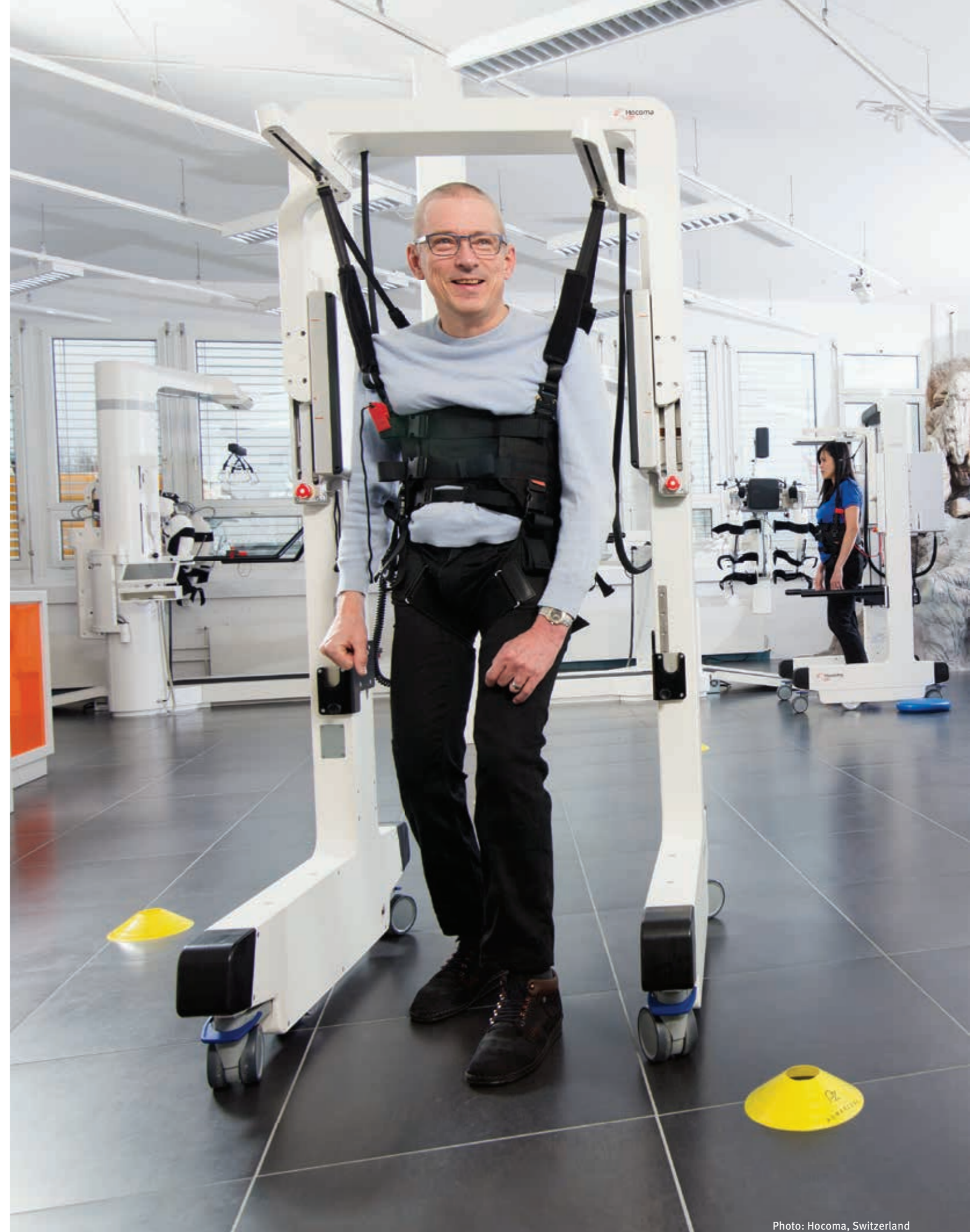
Andago is a mobile robot for body-weight supported gait training that allows upright, hands-free walking without spatial limitations.
